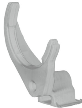
Aluminium Mold (Reconstructed 3D model by CT computing)
