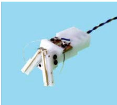
**Figure 6 – Four-Terminal Probe**
